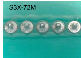
→ few flux residue cracks
