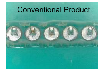
→ major flux residue cracking
